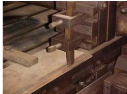
Fig. 4.5.20 Mounting of cutting tools in planing machine
