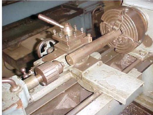
Fig. 4.5.10 Holding drill chuck and drill in tailstock.
