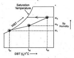
In this case, both cooling and dehumidification are carried out one by one. First, cooling is done by passing refrigeration inside the coil tube. During this time, dry bulb temperature decreases from  $t_{\rm d1}$  to  $t_{\rm d3}$  but specific humidity is constant. Then, dehumidification is done by removing moisture from air. Due to this, SP; humidity decreases but DBT remain constant.
